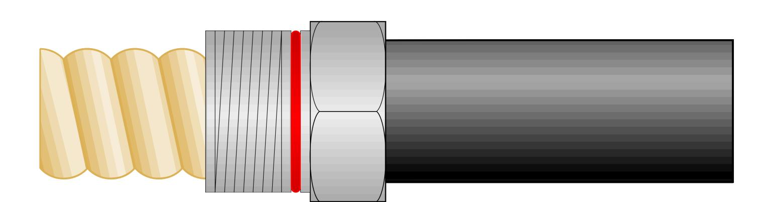
Using a sharp knife, cut the cable screen and foam dielectric flush with the body of the locking nut
